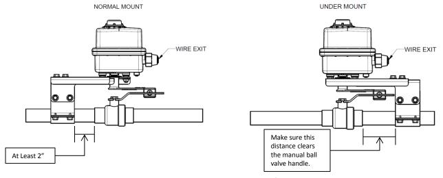
Make sure the pipe and valve are at least two inches from any obstruction such as a wall. Ensure there is a power source within 6 ft. of the Clamp-On Actuator.
